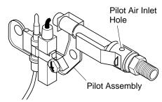
Figure 21 - Pilot Inlet Air Hole
